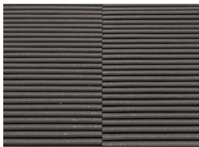
Before: Imperfect rib alignment.
