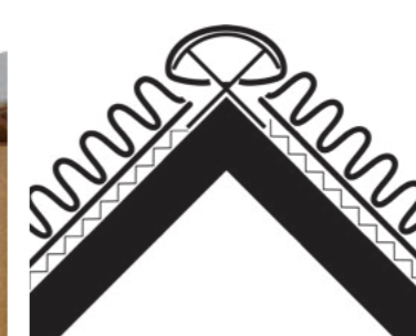
A corner profile can be wrapped in matching leather to create a more robust corner junction.
